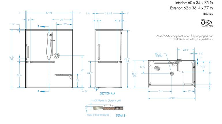
FEATURES Dimensional Tolerance ± %". Dimensions needed for site preparation should be measured from the unit. Aquatic assumes no responsibility for preparatory work.
