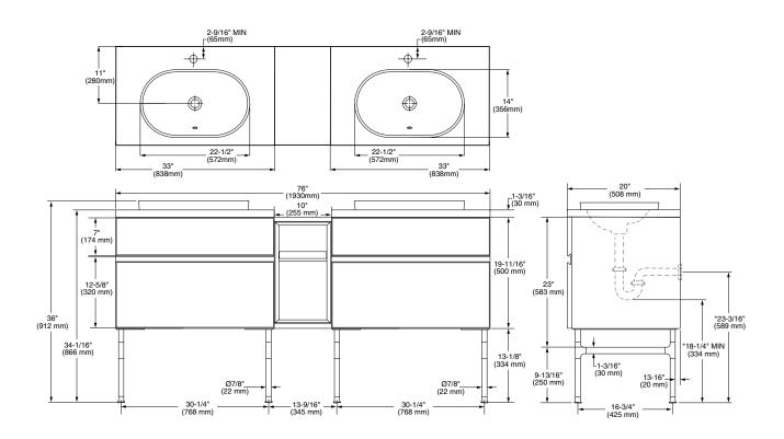
NOTE: Vanities can be installed with optional vanity leg set shown or mounted directly to wall.
