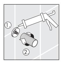
Cut the slip coupling so that it extends ½" outside the surface of the finished wall.
