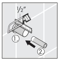
Cut the extension spindle so that it extends  $1\,{}^{1}\!{}^{4}$  " outside the surface of the finished wall.
