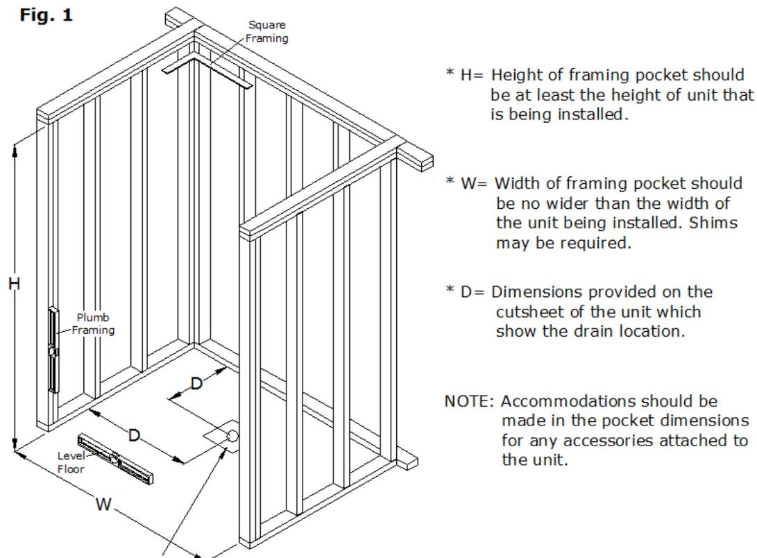
8" x 8" or 8" Dia. Core at least 2" deep must be drilled on center with the drain to permit the drain area to be pulled down by the plumbing connection. The drain must be aligned in the center of the core to insure proper installation and drainage slope.
