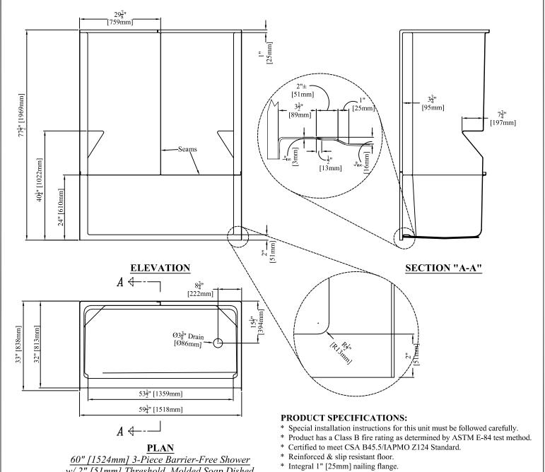
w/2" [51mm] Threshold, Molded Soap Dished, & Left or Right Hand Drain
