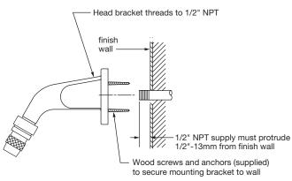
5-3/4" 3-1/8" 146mm 79mm 3" 76mm (H) 3-5/81 92mm turn knurled cylinder for adjustment
