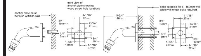
Anchor plate used for ceramic tile application-plate screws to wall and tile is applied up to sides of plate. Mounting bracket is mounted on finished wall with machine screws into anchor plate
