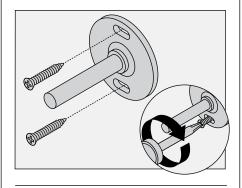
4) Slide accessory into position on bracket and secure with set screw.
